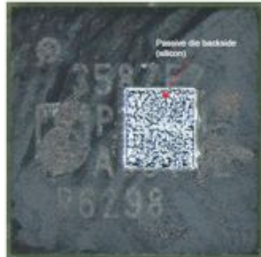
Laser decapsulation: Plastic etching down to passive die backside (silicon).
