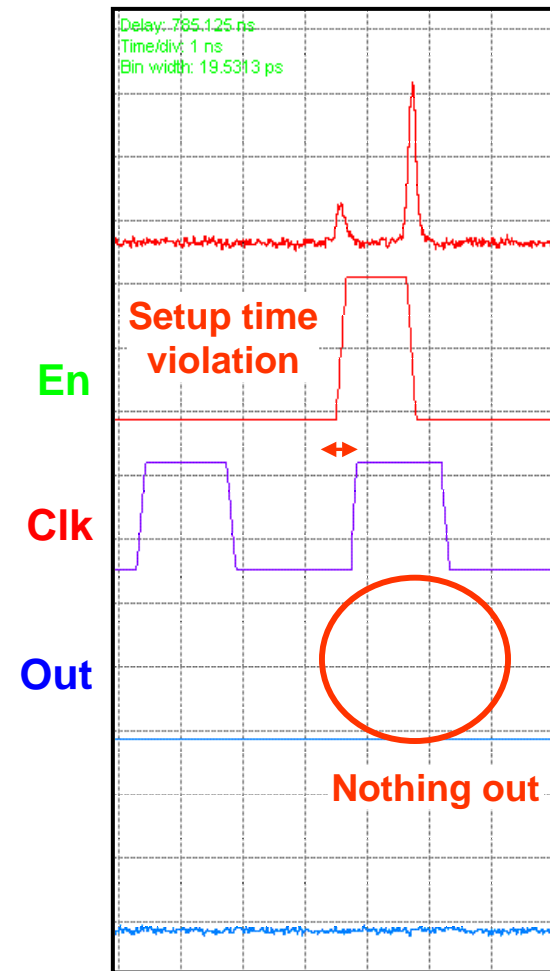
Fail @ 1.30v 290 MHz
