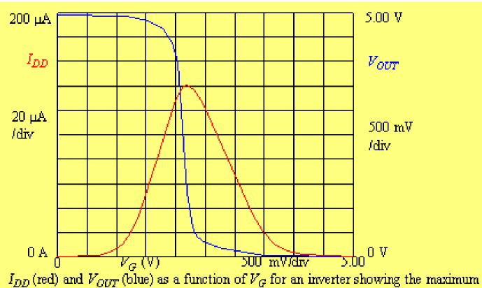
emission regions for the n and p-channel transistors.  $V_{OUT}$
