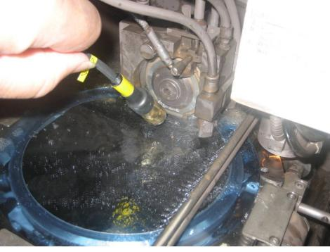
Using a new developed Trek measurement head for humid environment measurements, it was found, that the surface voltage of water drops may reach some hundreds of volts
